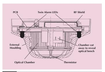
Fig.15 Sectional view - XP95 Multisensor Detector
